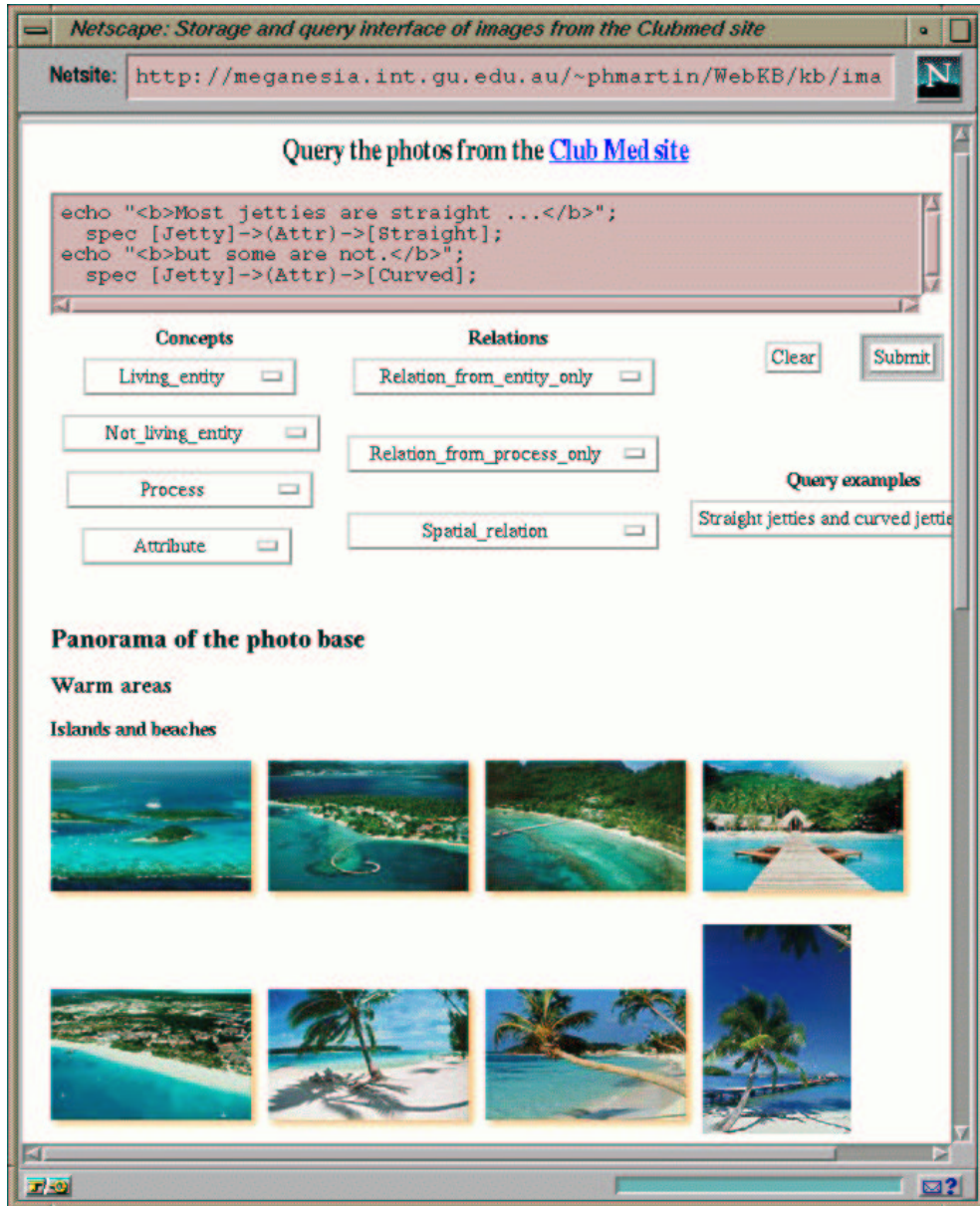
Fig. 5. Images, knowledge indexations and a customized query interface contained within a same document (the example query shows how the command "spec" which looks for specializations of a CG can be used to retrieve images indexed by CGs. The results are shown in Figure 6)
